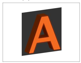
formed objects (of metals) with lighted fronts. special profile for holding fronts ('Elkamet', 'f-signTrim'etc)
